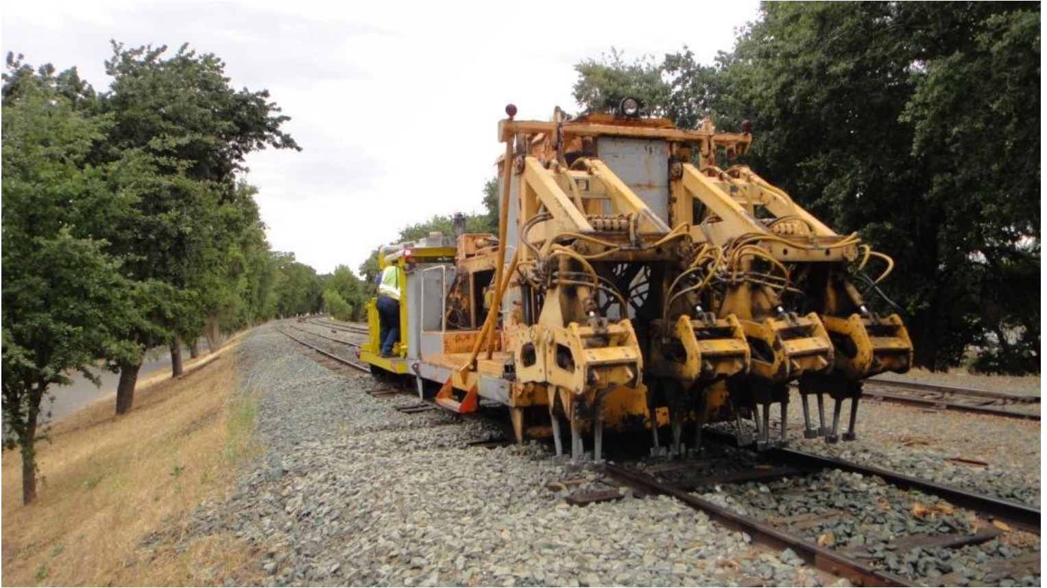
Hospital train headed back to town: with brakes released, the old-old tamper is towed back to town by the tug
